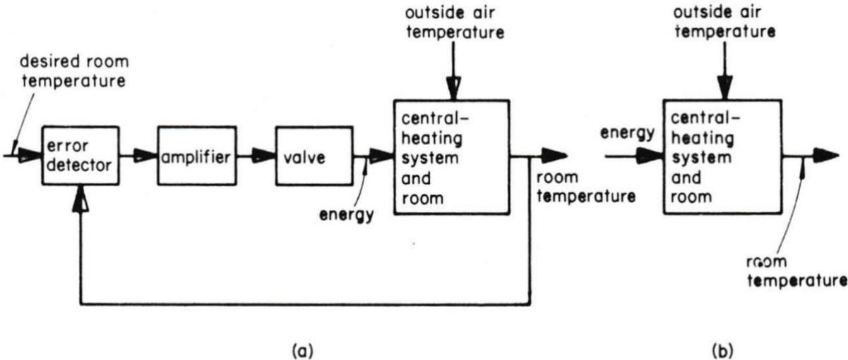
**Figure 2:** A central-heating system at home [2]
