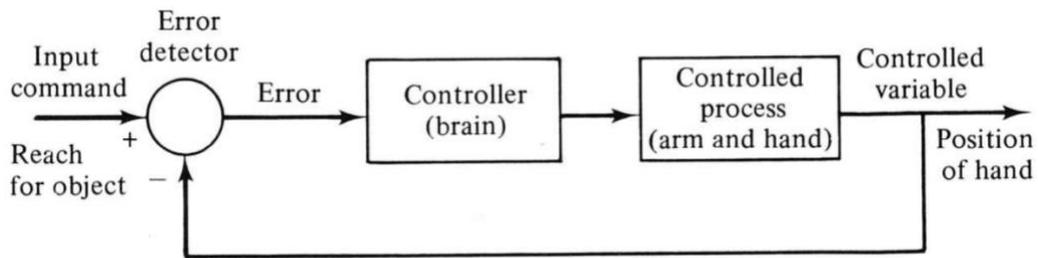
**Figure 4:** Block diagram of a human being as closed-loop control system [1]
