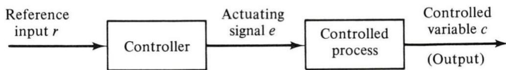
**Figure 3:** Block diagram of an open-loop control system [1]
